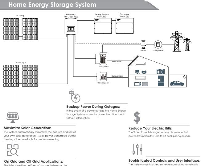
The Integrated Home Energy Storage System can be configured to operate in On-Grid and also Off-Grid scenario.
